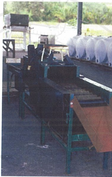
Figure 2.4 An automatic noni fruit washer, adapted for use with noni from a vegetable operation (Anonymous, 2002).
