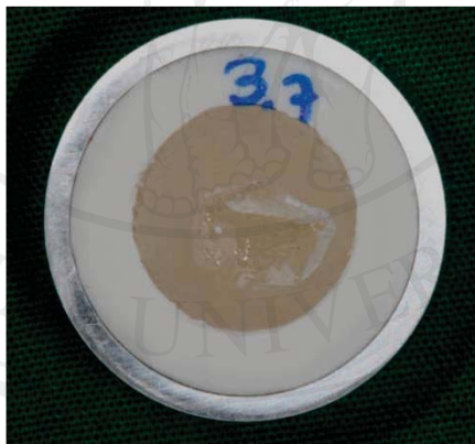
Figure 5.1 Porcelain specimen with surface fracture
