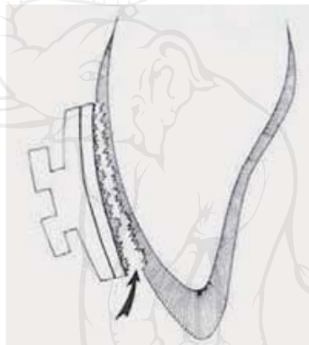
Figure 4.5 Cohesive failures within porcelain 38
