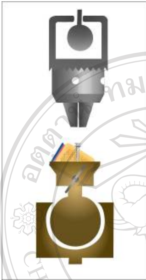
Figure 5.5 A custom-made base to hold the specimens and a grip to grasp the miniscrew head were specially designed to allow a controlled angle to the axis of the pull.
