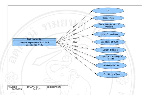
Figure B.14 Internal Inspection of Main Tank Knowledge of PT.
