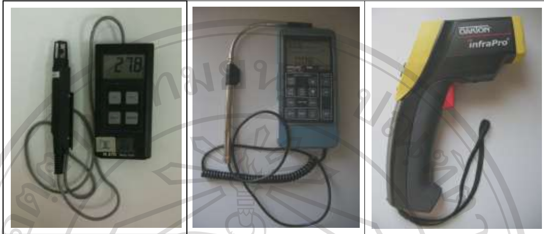
Figure 3.2 Two types of thermometers sensor, and a thermo gun
