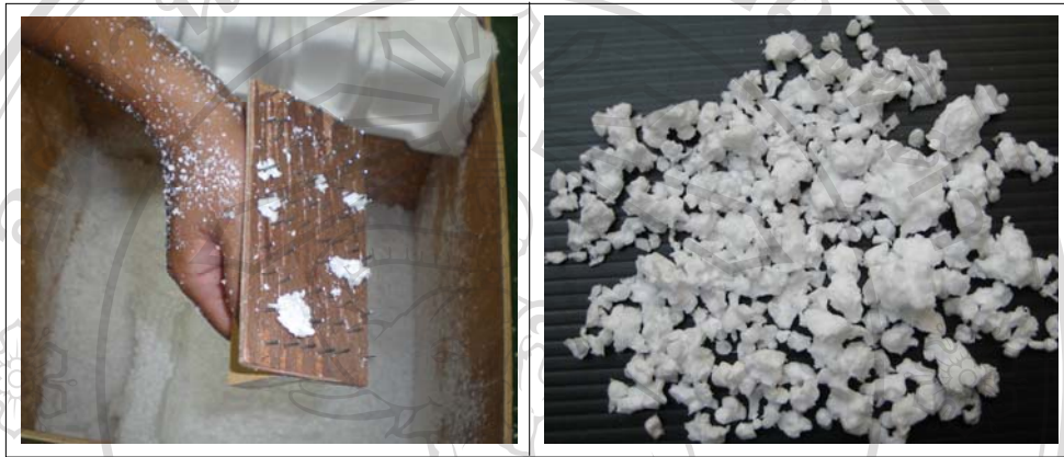
Figure 4.2 Scratching packaging foam by nail pad yields a mix-particle size 0.1-15 mm
