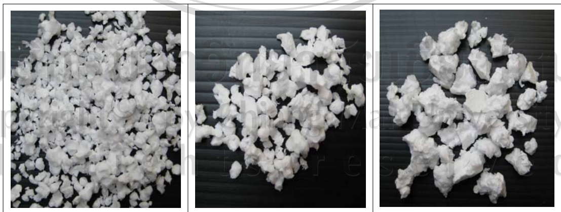
Figure 4.3 Packaging EPS particles (from left to right) Size 0.1-6, Size 6-10 and Size 10-15
