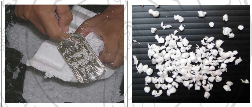
Figure 4.1 Shredding packaging foam by papaya shredder yields particles size 0.1-3 mm
