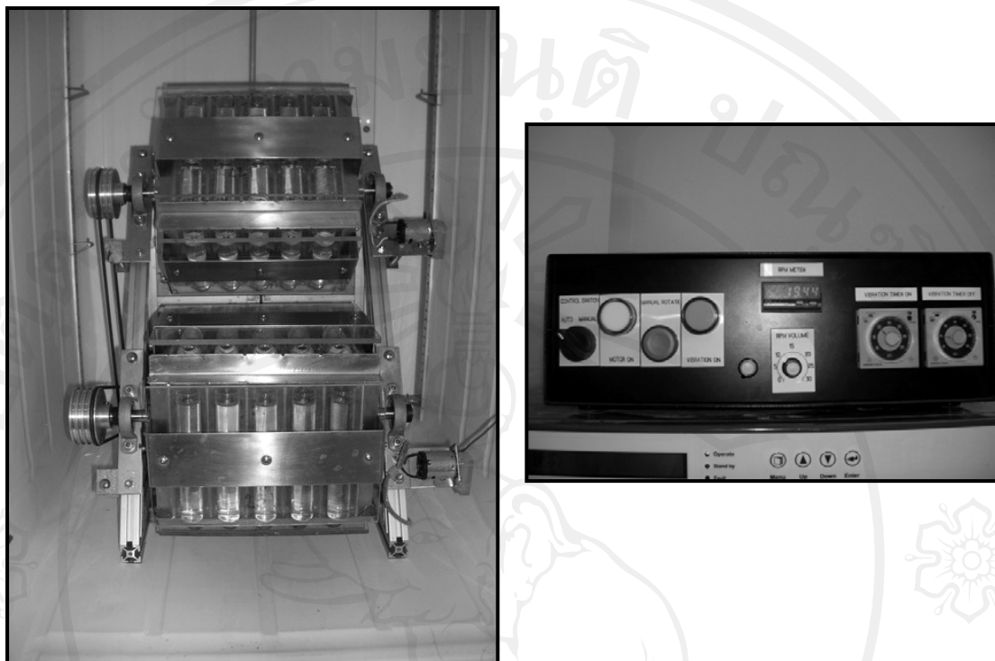
Figure 3.2 The biotransformation bottle was placed in a rotary tumbler mixer at 10 rpm, 4°C for 72 h
