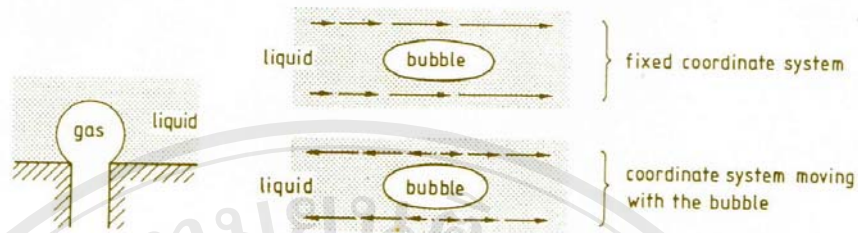
Fig. 2.1(right) Deformation of gas bubble subject to extensional flow by the surrounding liquid (Dickinson and George, 1988).
