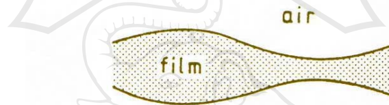
Fig. 2.4 A disturbance of a liquid film in the form of a symmetric wave (Dickinson and George, 1988).
