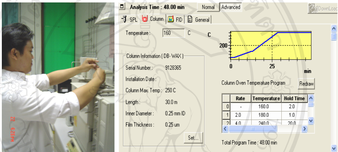
Figure 15. Fatty acid analysis by Gas chromatography (left), Condition control by computer program (GC solution) (right).
