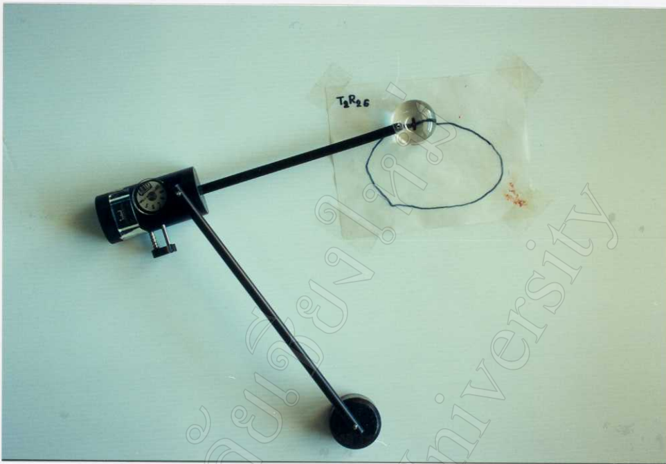
Figure 22 Using Planimeter to measure loin eye area.
