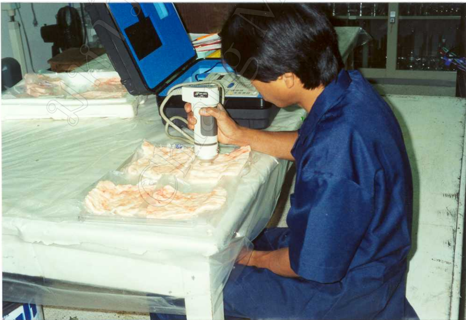
Figure 16 : Measurement of perirenal fat color by Minolta chroma meter
