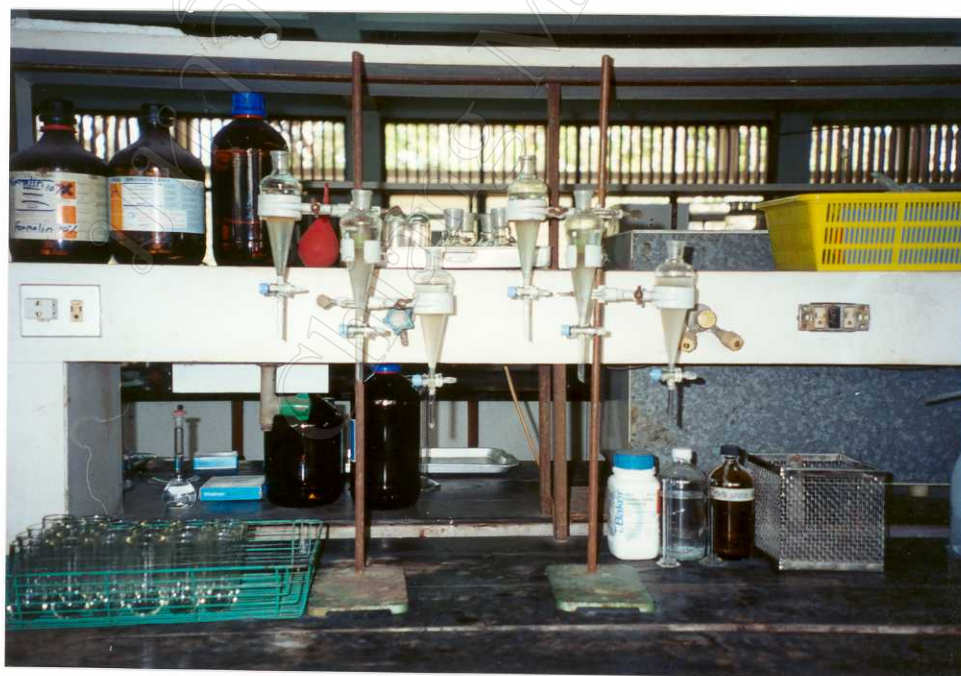
Figure 20 : Separation of oil in solvent (chlorofom : methalnl, 2:1) by separating funnel
