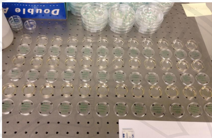
Figure 3.6 Various PS Petri dish with PBS immersed for the release rate detection.
