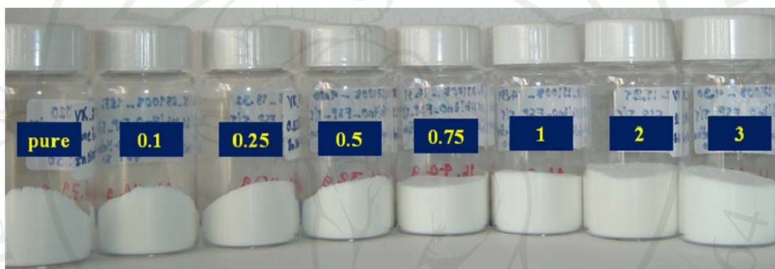
Figure 2.6 The flame-made (5/5) pure ZnO and 0.10-3.00 mol% Nb-doped ZnO nanoparticles ordered from the left to right with increasing Nb concentrations.
