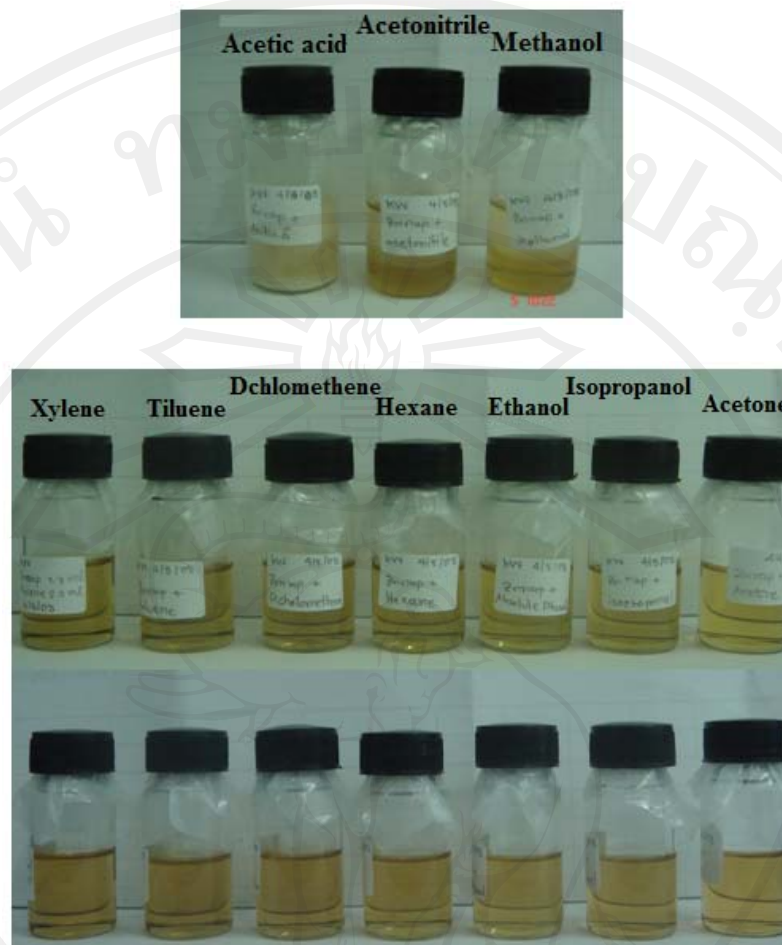
Figure 2.1 The solubility tests of the precursors were performed using zinc naphthenate as a Zn precursor dissolved in several organic solvents prior to the precursor preparation.
