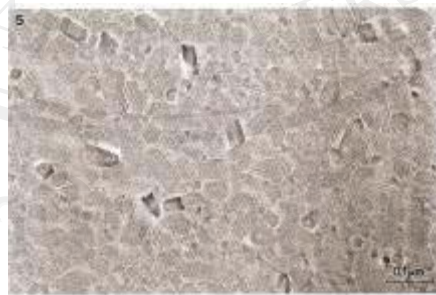
Figure 2.5 Transmission electron micrograph of cross-cut crystals obtained from the highly mineralized surface layer. Large flattened hexagonal crystals are scattered throughout the section, and many extremely small, irregularly-shaped crystals can be observed among them. 15
