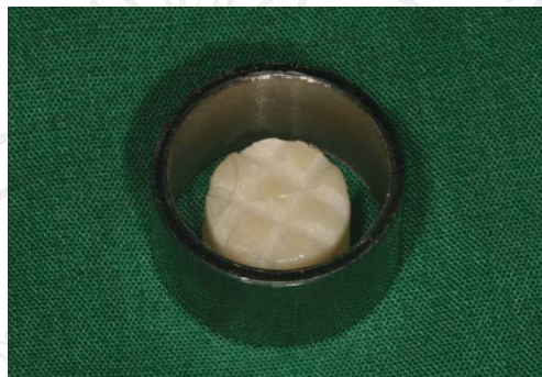
Figure 3.13 The surface of the porcelain disk was exposed parallel to the rim of the ring (bottom surface)
