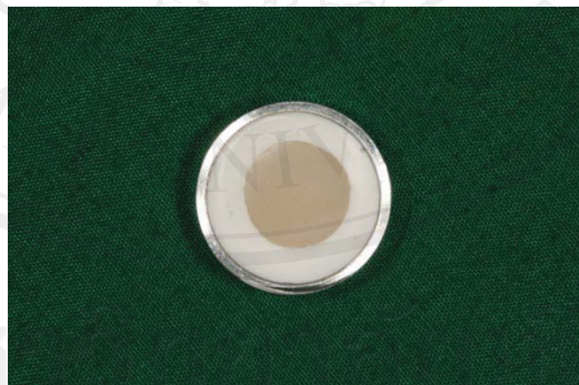
Figure 3.14 Porcelain specimen - embedded disk with self-curing resin in stainless steel ring
