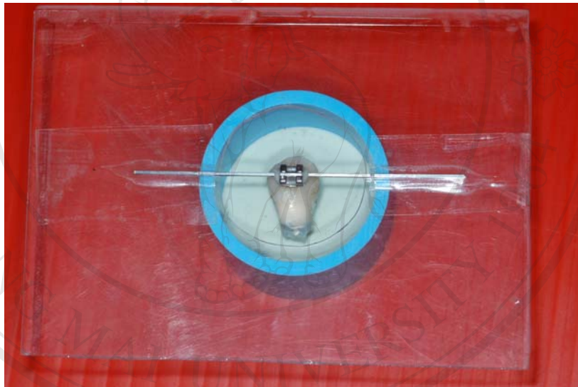
Figure 3.11 A 0.018" X 0.025" stainless steel wire was placed on the bracket slot by ligating the elastic ligature to the body of the bracket.
