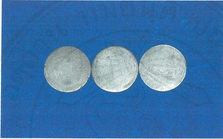
Figure 3.1 Magnet specimens in the dimension of 20 mm in diameter and 2 mm in thickness
