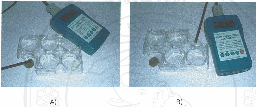
Figure 3.8 The measurement of single magnetic field at two positions of culture plate: A) the position 1 was the closest to the magnet, B) the position 2 was the farthest from the magnet.
