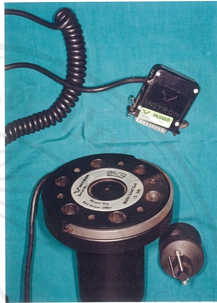
Figure 20 a. Instron ® universal testing machine b. Five kilonewtons load cell
