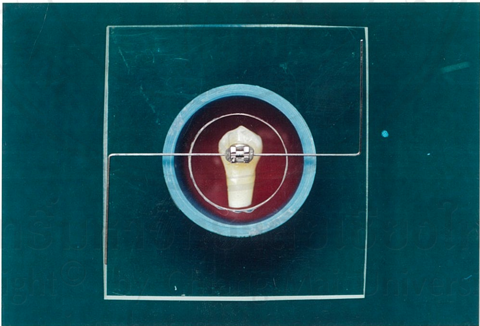
Figure 28 The 0.018" x 0.022" stainless steel wire ligated to tooth-bracket assemble with elastic ligature was placed above the polyvinylchloride (PVC) block 2 millimeters by the thickness of plastic plate
