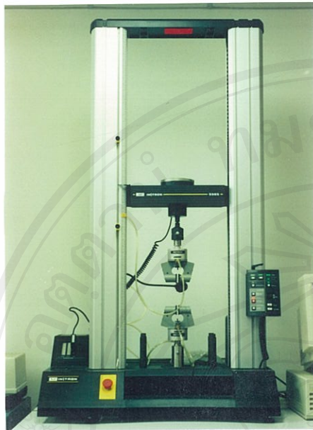
Figure 20 a. Instron ® universal testing machine b. Five kilonewtons load cell
