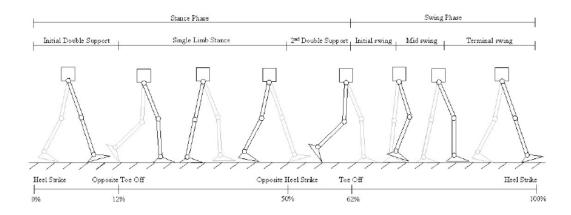
Figure 1 Human walking gait through one cycle, beginning and ending at heel strike. Percentages showing contact events are given at their approximate location in the cycle (25)
