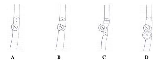
Figure 2 Orthosis knee joint often used in KAFO. (A) Single-axis knee joints (B) Single-axis locking knee (C) Offset knee joint (D) Variable position orthosis knee joint (69)
