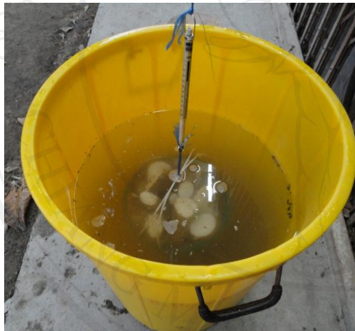
Figure 8 Measurement of starch content; (A) sample preparing (5 kg), (B) weight sample in water and (C) reading the sample weight.
