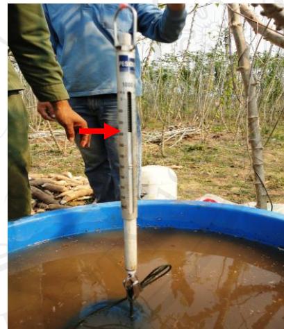
Figure 8 Measurement of starch content; (A) sample preparing (5 kg), (B) weight sample in water and (C) reading the sample weight.
