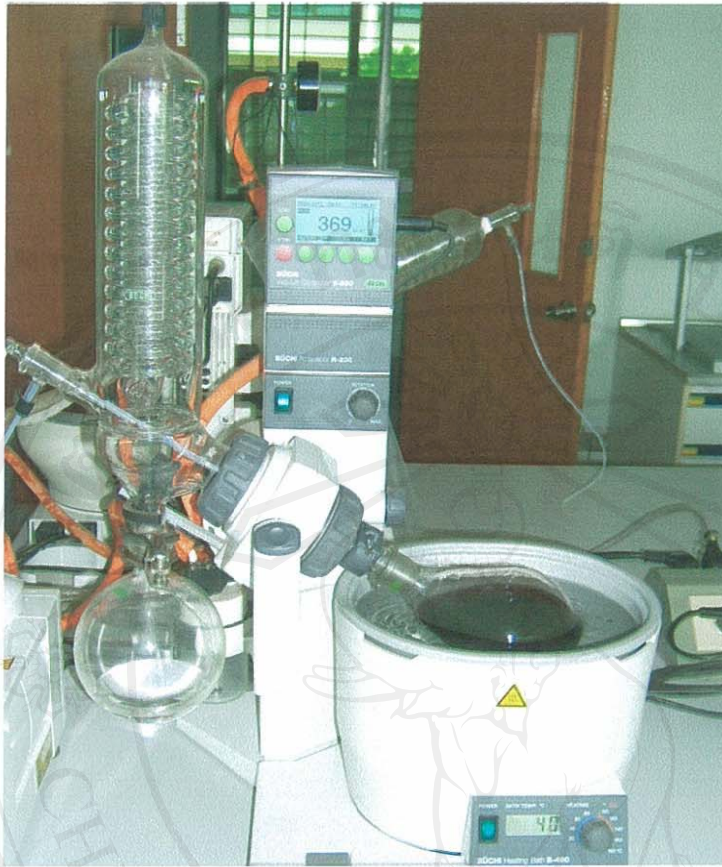
Figure 3.3 The 70% acetone was removed by evaporator (Central laboratory).
