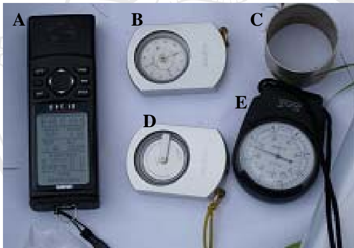
Figure 19. Data collection devices; A = GPS device, B = compass, C = metal pipe used for bulk density soil sample collection, D = clinometer and E = altimeter.
