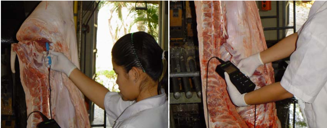
Figure 14. Measurement of pH-value on muscle.
