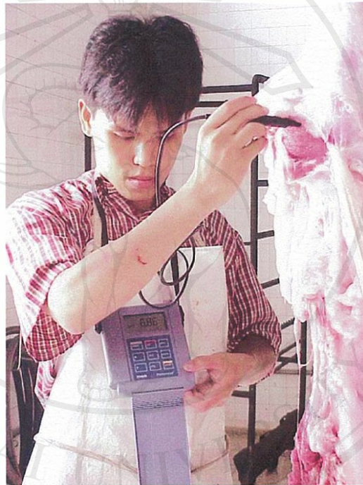
Figure 4 pH measurement at semimembranosus
