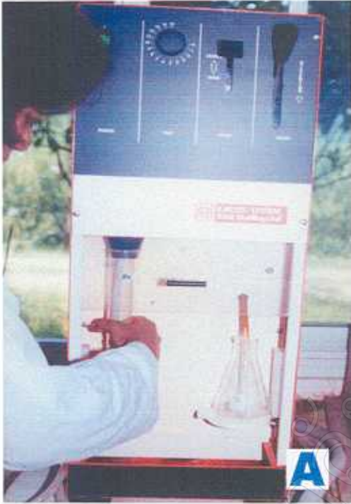
Appendix figure 10 Kjeldahl extraction (A) and Warner – Bratzler shear measurement (instron machine) (B)
